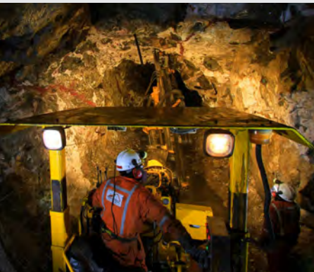
Jumbo drilling at Level 12 at Animas Vein
