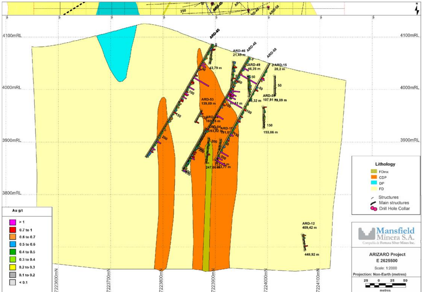
Figure 10.8 Section B-B' displaying mineralization at the Arizaro Deposit
